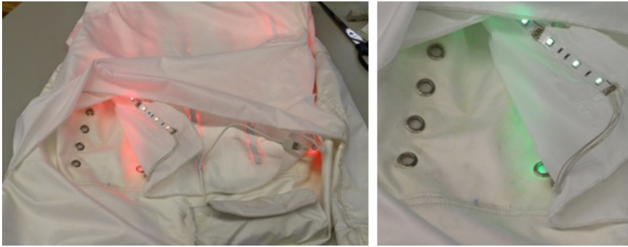
Figure 2: Jacket's interior (Left: Overview, Right: detail of ferrules and connections)
